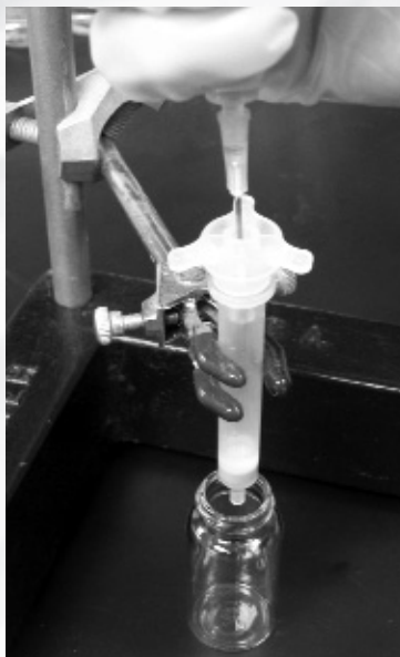
Figure 3. Introducing a solution to the column. Use a syringe with needle to pass the solution through the hole in the Luer adaptor.
